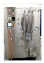
EmulsiFlex-D20 Capacity: 20 L/h Pressure: up to 2000 bar Min. sample volume: 50 mL Air pressure: 8 bar
