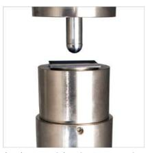
in the ASTM D7136M, ASTM D7136, machine performs the impact of a guided striker perpendicular and centered on the specimen. The tup The first step is using a drop weight or striker insert has a hemispherical striking insert with a suitable diameter (e.a. 20 mm) and tup holder can be equipped with additional weights. Round or square specimens, clamped pneumatically activated clamping ring with a suitable diameter (e.a. 40 mm), are used.
