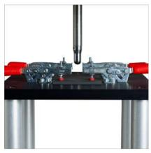
The CAI test procedure is described A drop weight impact testing ISO 18352 & Airbus AITM 1.0010 standards.
