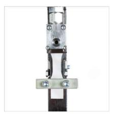
A tensile impact test measures the toughness of polymers using an impact tester for plastic according to the ISO 8256 standard. Polymers that are too flexible or thin for a Charpy or Izod impact test generally require an uniaxial tensile impact test with a relative high strain rate. The Instron impact test apparatus can reach a wide range of impact velocities from relatively low (0.7 m/s) to very high (22m/s).
